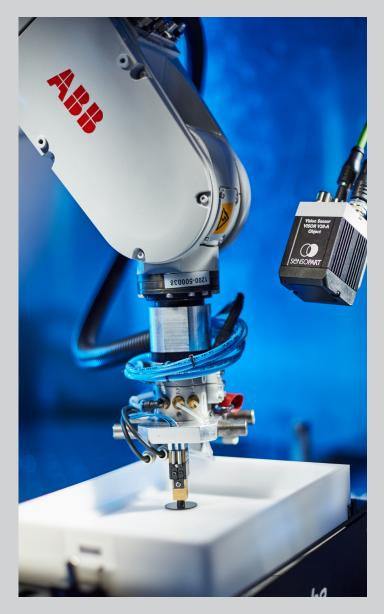
**1.The problem: distorted images in sensor coordinates** The robot cannot interpret sensor image pixels, which may also be inaccurate due to a diagonal angle of view and lens distortion.
