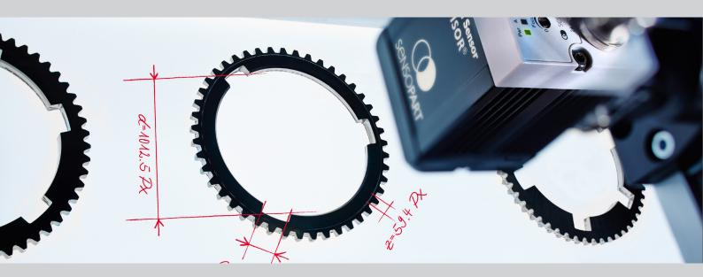
Component position and distance values are generally required in metric units, such as millimeters or inches, rather than in pixels. Thanks to the VISOR® calibration function, vision sensor coordinates can now effortlessly be converted into real-world engineering units: place the calibration plate into the sensor's field of view, a single mouse click in the configuration program and it's done!
